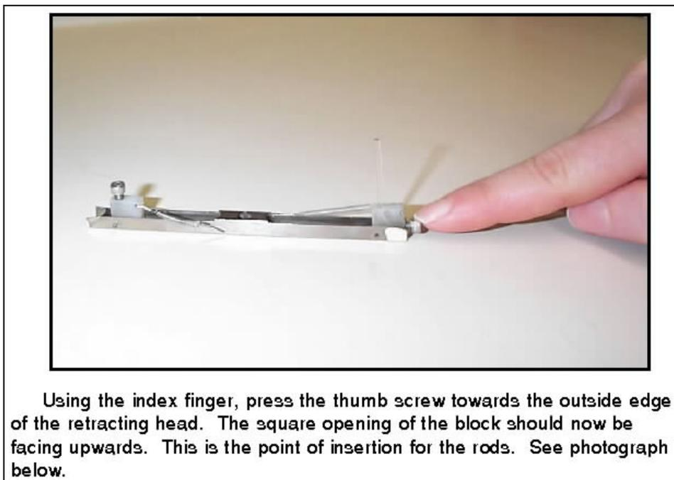
position with the thumb of the same hand. Hold the pivot block securely in the extended position while removing and replacing the rods. The marked faces of the rods should correspond with the LEADING
