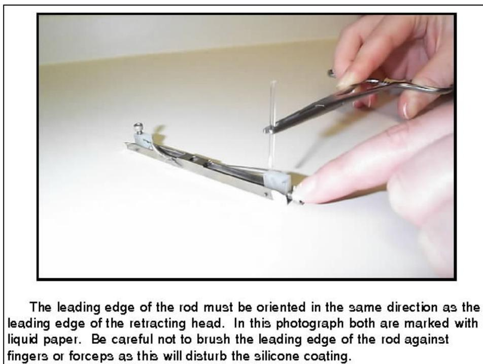
EDGE of the retracting head. We suggest marking the leading edge of the retracting head with nail polish or liquid paper to avoid confusion when replacing the rods. Gently press the rod in the square hole of the pivot block until it touches the metal flange of the head assembly.
